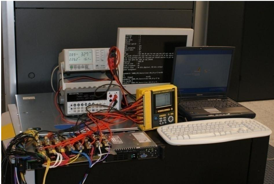
For each server a customized wiring and shunt configuration
