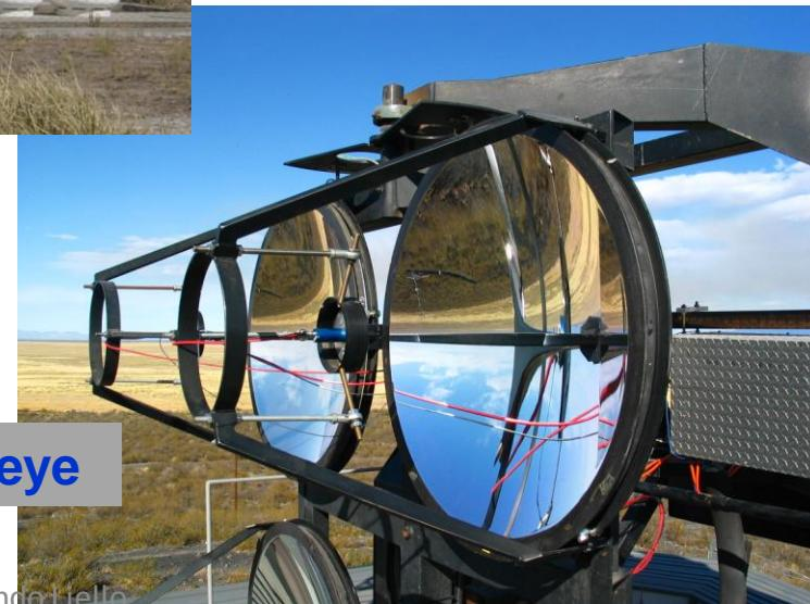
Lidar at each fluorescence eye
